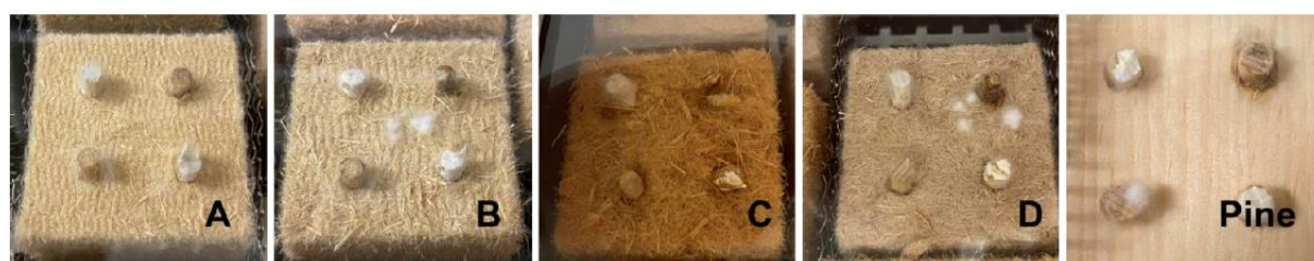
Figure 89. Visual observation after 8 weeks: established mycelium growth on all specimens apart from the flexible fibre mat C. p. 26
